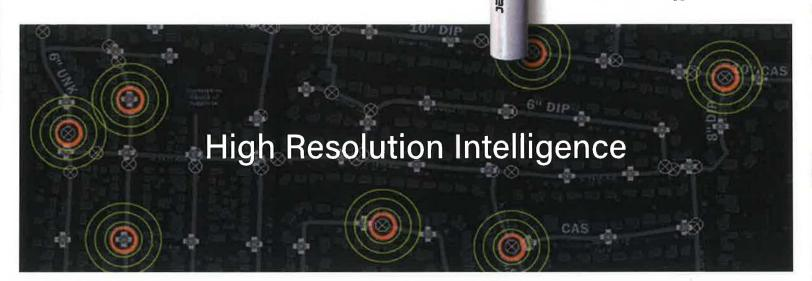
iTracker Smart Sensors deliver a network of high resolution data points that quickly pinpoint I&I down to a set of adjoining manholes.
