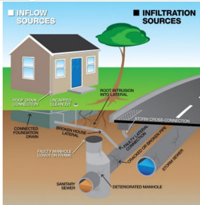
**Figure 1:** Typical Sources of I/I in Sanitary Sewer Systems
